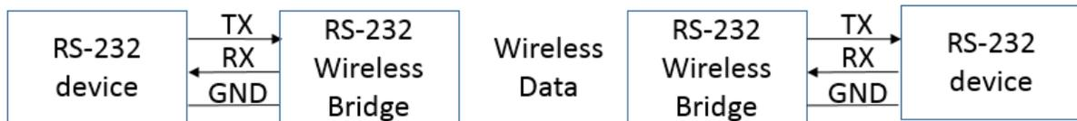
**Fig. 4 Typical RS-232 Point-to-Point Configuration**
